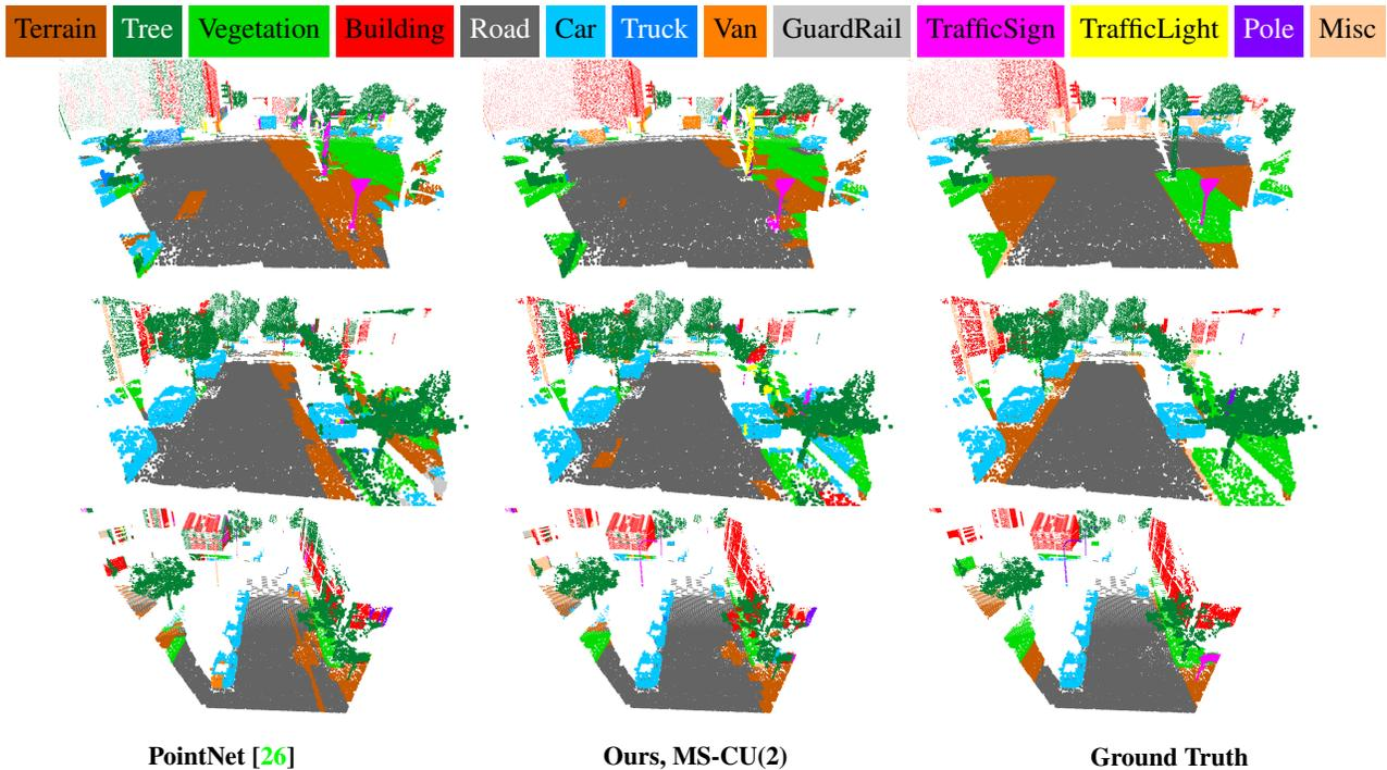
Figure 8: **Outdoor qualitative results.** Dataset: Virtual KITTI [8]. Results were obtained using only XYZ coordinates as input, no color information was used. Left: baseline method PointNet. Center: our results using the MS-CU model as illustrated in Figure 3. Right: ground truth semantic labels. The outputs of our method are less fragmented (cars, houses) and finer structures like street lights and poles are recognized better.
