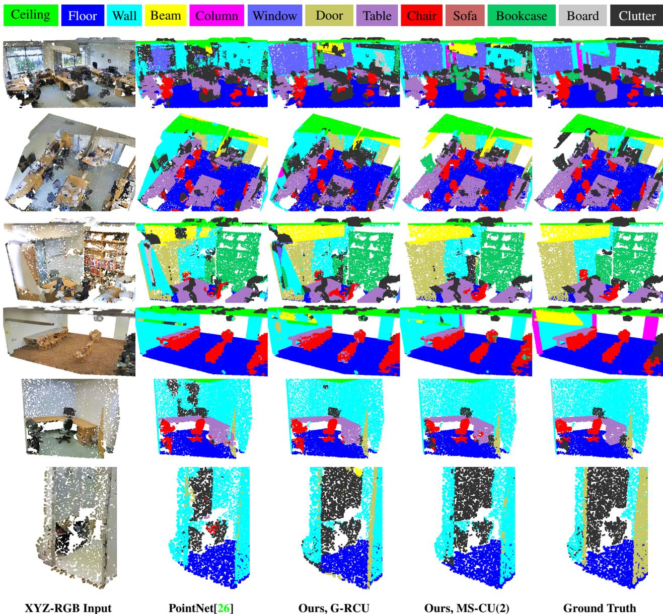
Figure 7: **Indoor qualitative results.** Dataset: S3DIS [1] with XYZ-RGB input features. From left to right: input point cloud, baseline method PointNet, our results using the G-RCU model (see Figure 4), our results using the MS-CU(2) model (see Figure 3), ground truth semantic labels. Our models produce more consistent and less noisy labels.
