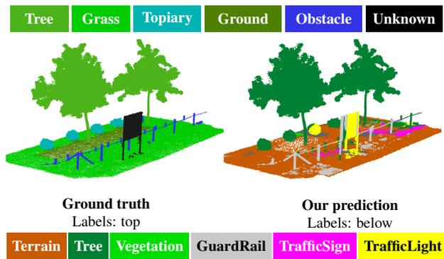
Figure 9: **Qualitative results on 3DRMS'17 Challenge.** We trained our model on vKITTI point clouds without color and applied it to the 3DRMS laser data. Training and test datasets do not have the same semantic labels. Despite that, common classes like trees are successfully segmented and plausible ones are given otherwise (e.g. terrain instead of grass, guardrail instead of obstacle).
